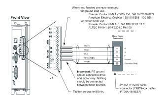
Figure 14: Epsilon Motor Power Wiring Diagram
